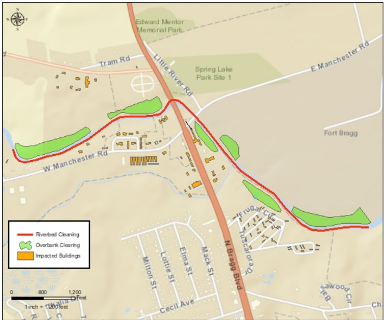
Figure 6-12 - Little River Riverbed Cleaning and Overbank Clearing (Section 2)
